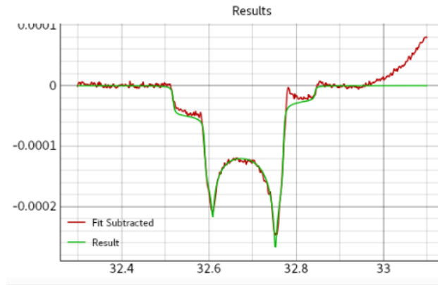
Figure 3: A deuteron polarization signal, showing a characteristic double NMR peak, after the extraction process. This illustrates the failure of the polynomial fit to completely remove the background drift for a small NMR signal, causing inaccuracy in the measurement.
