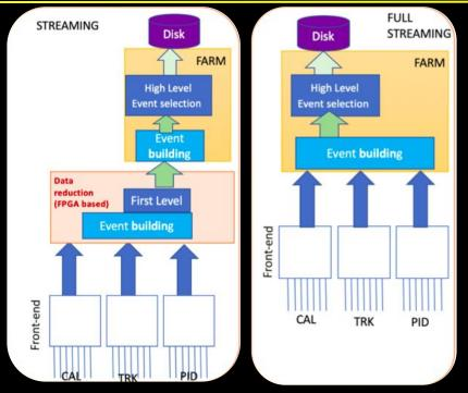
Different streaming pipelines: FPGA based (w/ data reduction) and full streaming. ML naturally suited for online data reduction or high level physics event selection/trigger
