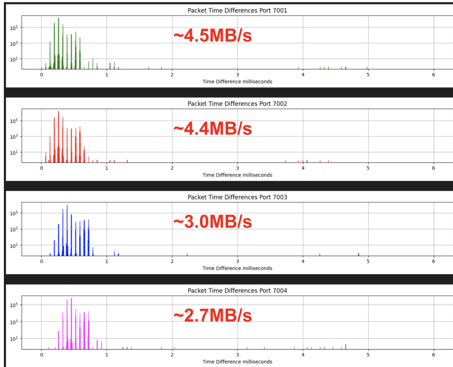
Figure 3: Time difference in milliseconds between packets arriving at ejfat-fs node in CEBAF center streamed from Hall-D DAQ system. The different plots/colors represent different destination ports.
