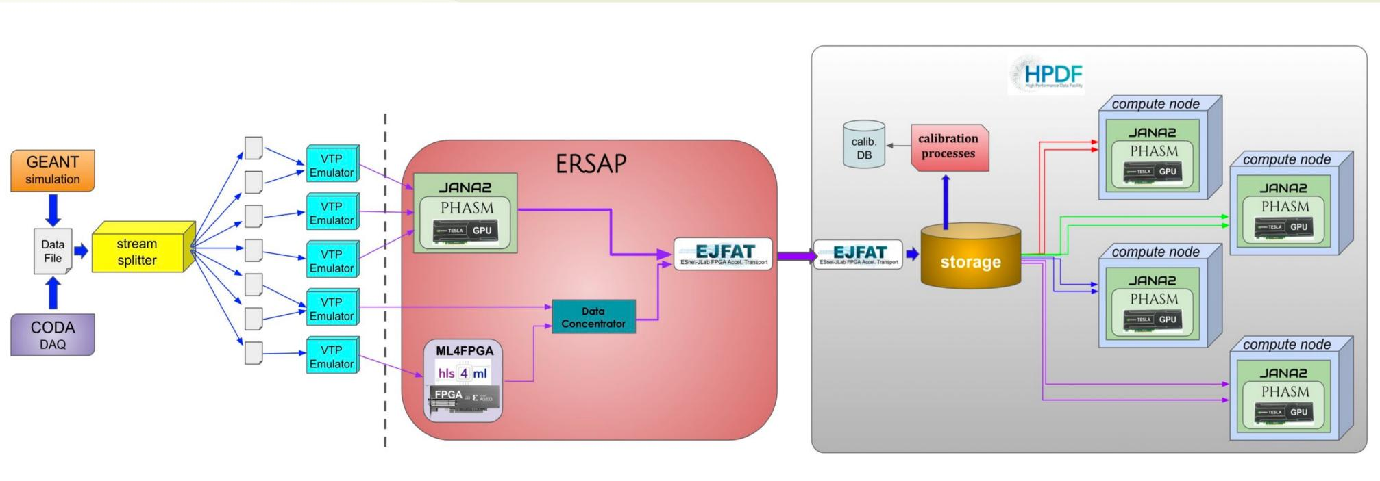
Highly configurable multi-stream source allows realistic streaming simulations
