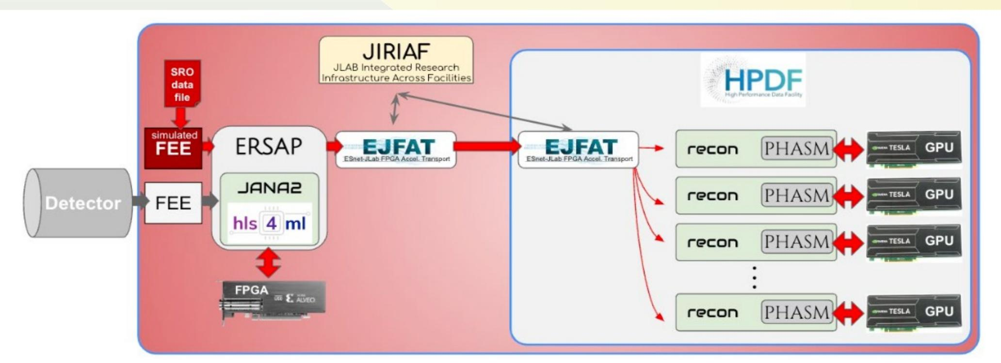
Diagram illustrating an example SRO system where data is streamed from the detector to
