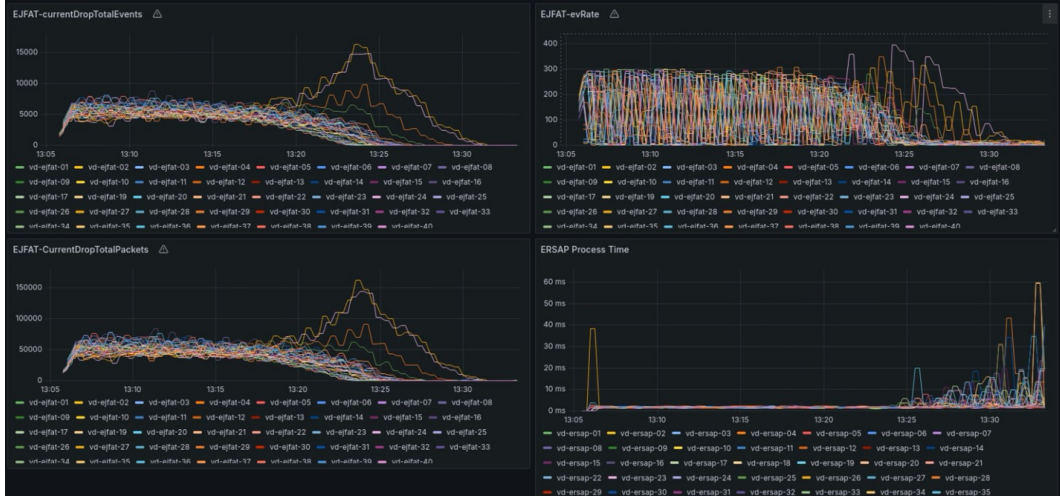
Figure 3: Monitoring system metrics scraped from applications during the JIRIAF deployment. The figure shows the metrics collected by the monitoring system, providing insights into the performance and resource utilization of the deployed CLAS12 event reconstruction application across the NERSC cluster nodes. These metrics are crucial for evaluating the effectiveness and efficiency of the JIRIAF framework in a high-performance computing environment.
