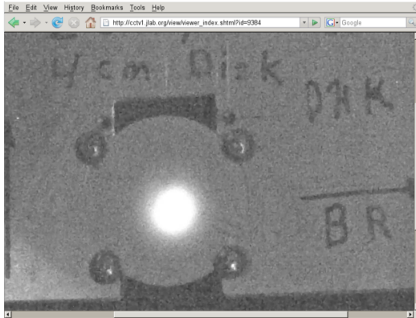
Figure 3: Beam spot on the tagger dump viewer.
