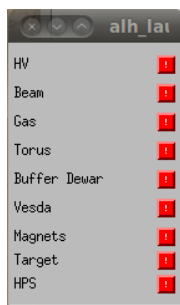
Figure 5: Hall B controls screen for launching alarm handlers for individual subsystems.
