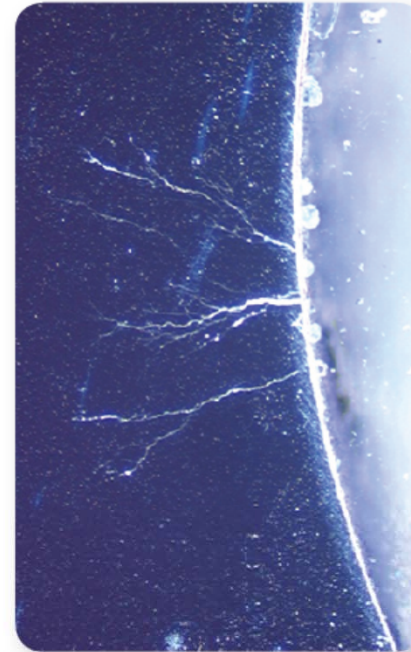
Cracking Thresholds are measured by exposing pre-cracked samples to tritium gas and slowly pulling them apart or by step-loading and holding until crack begins to grow. Crack growth is monitored by using the DC-Potential Drop technique.
