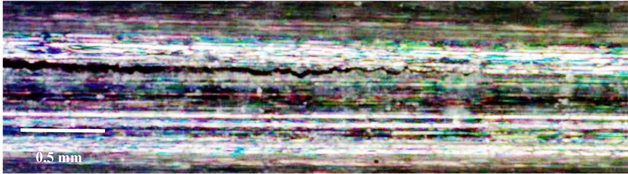
MM75-2, K = (20.3 \text{ MPa}\cdot\sqrt{\text{m}}) , 4 month exposure
