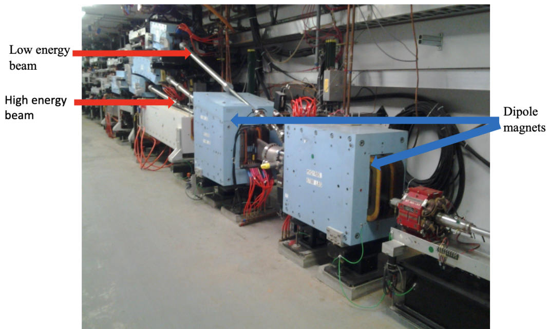
FIG. 4. A photograph of a recombining system at the beginning of South linac.
