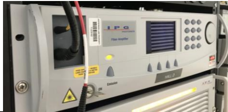
High Power (6 W) 1560 nm Fiber Amplifier
