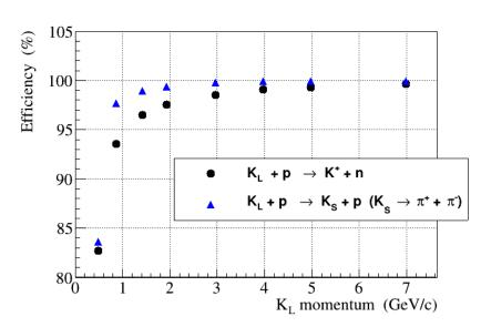
Trigger efficiency 1.5 GeV/c  $< P_{KL} > 4.5$  GeV/c
