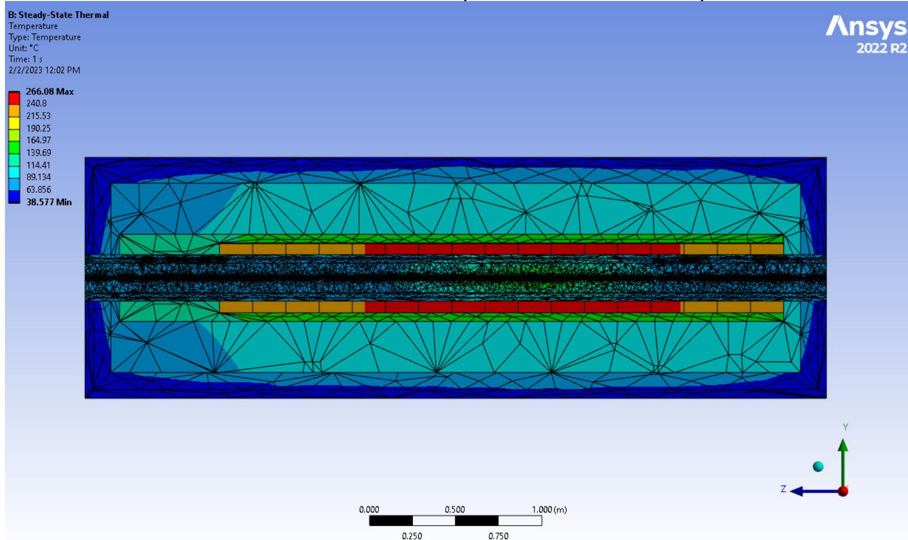
Cu extended to end, 7cm wide, 100 micron air gap between bodies, finer mesh on cu, no W
