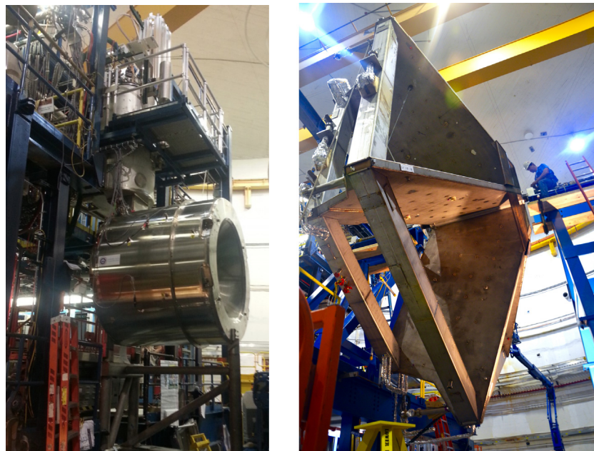
Fig. 4. The CLAS12 magnet systems. Left: The fully assembled solenoid magnet including all cryogenic connections on the beamline at the beginning of cool down, before the detector installation. Right: The torus magnet with all six coils mechanically assembled in a common cryostat. The coil cryostat, which is fabricated from non-magnetic steel, has an outside width of 124 mm. The cross bars provide a cold (4.5 K) cryogenic connection of neighboring coils, and counteract the out-of-plane forces to provide mechanical stability to the full magnet. Due to the large physical size of the assembled torus magnet, the final assembly of the magnet had to be completed in Hall B.
