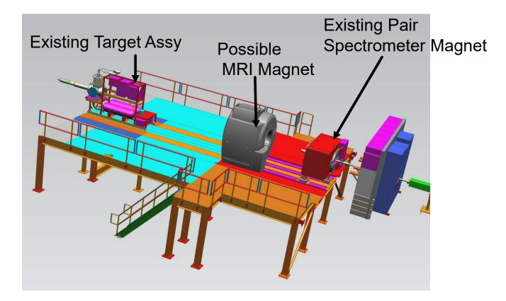
Proposed MRI Magnet can fit in existing space and platform can support the weight
