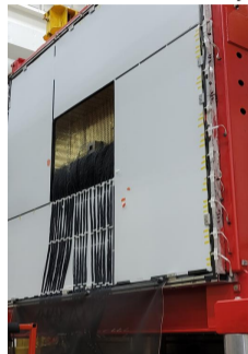
Installation of the bases for crystals and cabling
