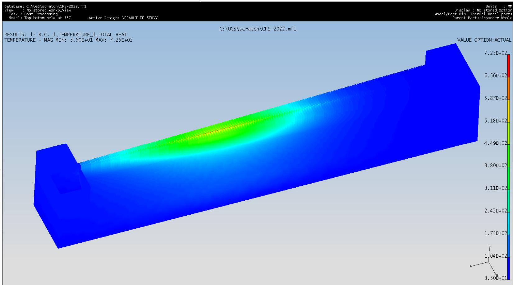
40KW total power using 3mm hole and distribution scaled to Hall C over 50 cm
