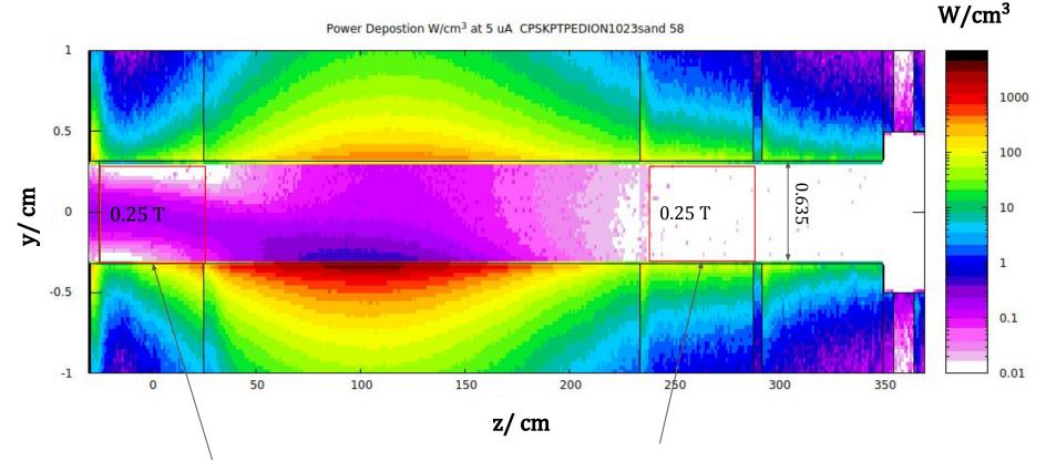
• Upstream magnet forms the Hot Spot; Downstream - cleans the photon beam.
