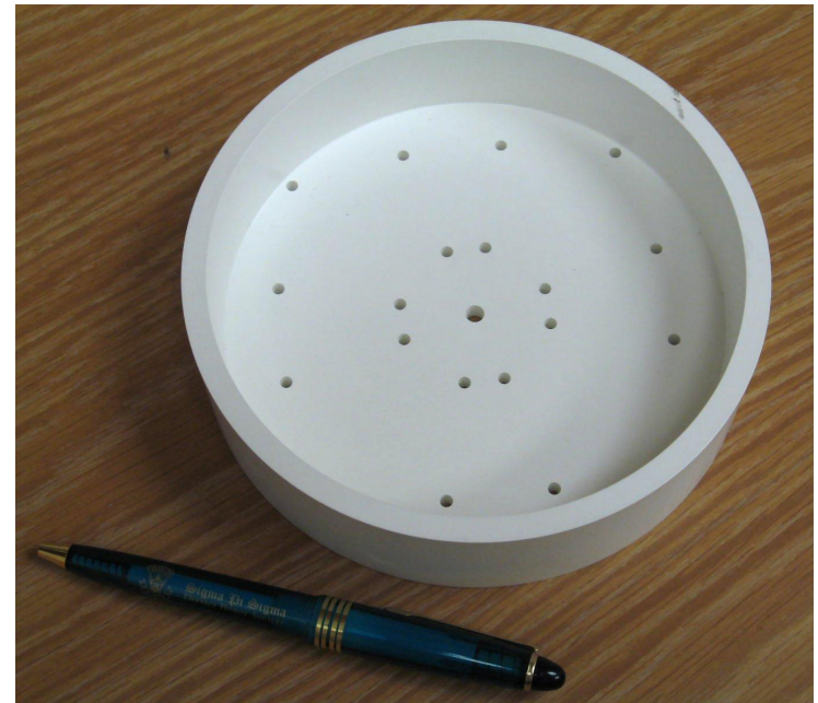
insulating cathode holder (BN)
