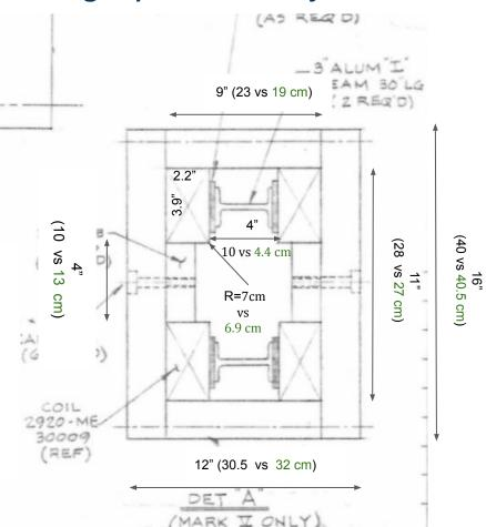
Coil 122 windings 20 kA-turns vs 1.8 kA\*16 = 29 kA-turns
