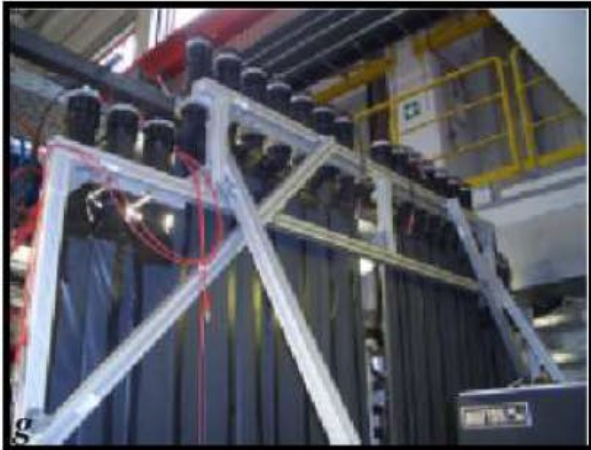
Figure 3.24: Installation of the new FVH layer: First the element is put on the lower holding system, which holds the weight of the element (a). After that the upper part is attached (b, c) and both clamps are fixed. The exact position of the upper clamp is not fixed to allow tolerances in the length of the element. Photo d) shows the first two installed elements, photo e) the elements at the beam pipe. Photo f) shows
