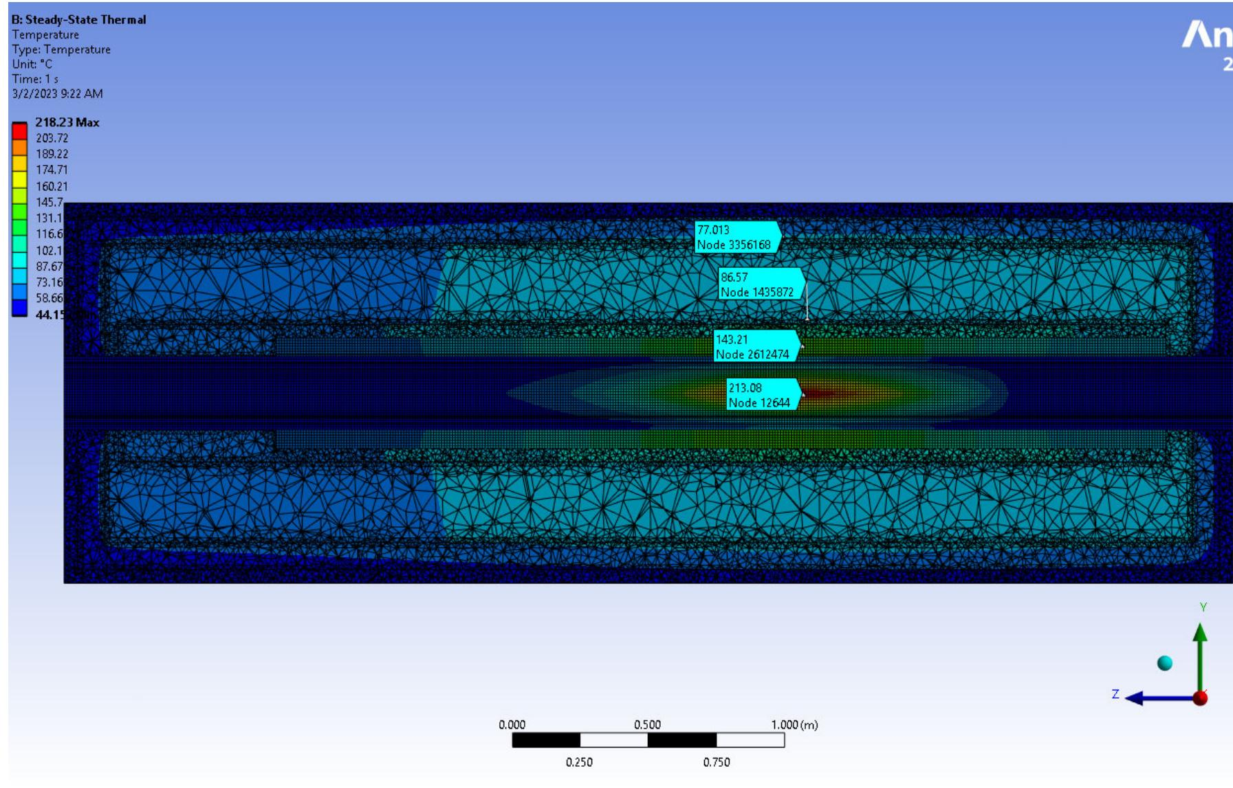
Coarse mesh, 1cm elements, 51KW heat, 1 mm air gap between each material, Cu->steel->tungsten->lead->poly->lead
