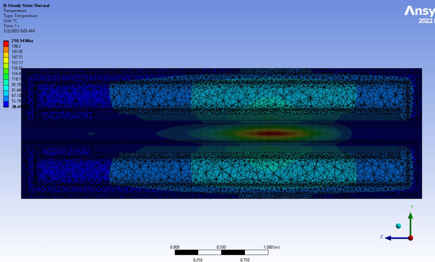
Coarse mesh, 1cm elements, 51KW heat,
