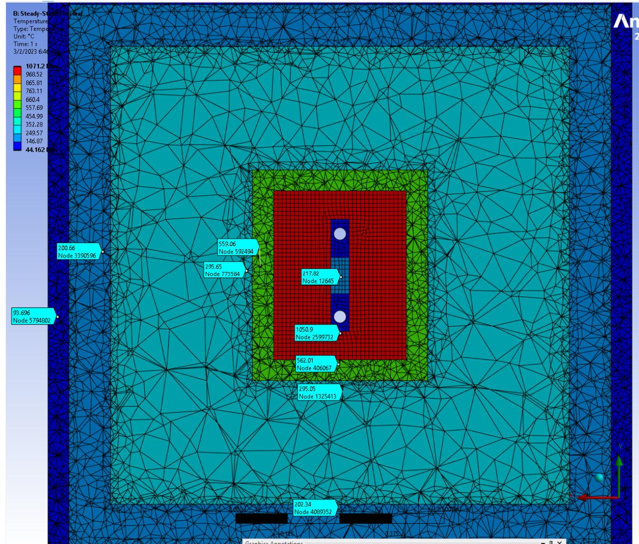
Coarse mesh, 1cm elements, 51KW heat,
