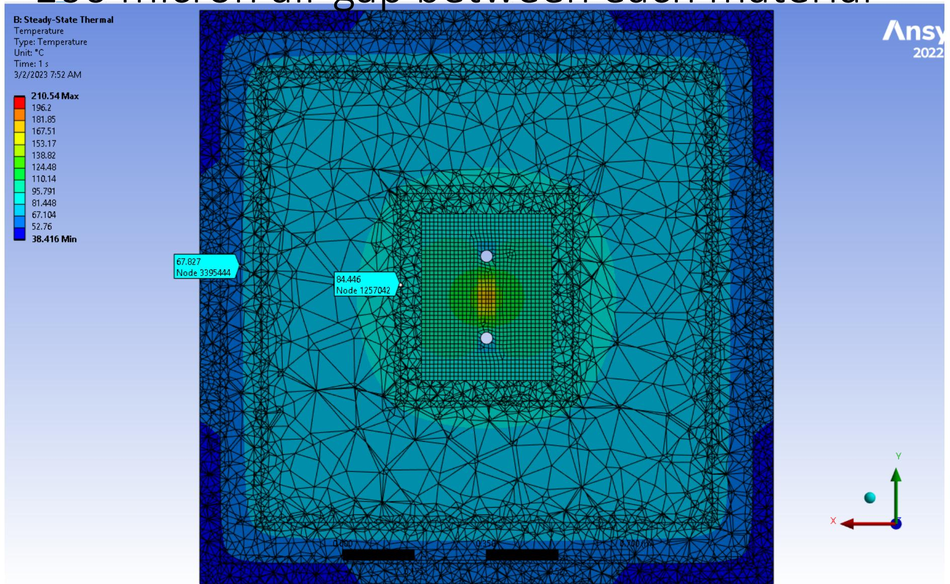
Coarse mesh, 1cm elements, 51KW heat,
