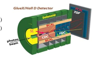
• Trigger algorithm based on measurement of energies in FCAL and BCAL
