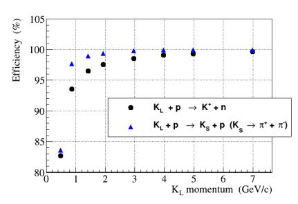
Trigger efficiency  $1.5 \text{ GeV/c} < P_{KL} < 4.5 \text{ GeV/c}$
