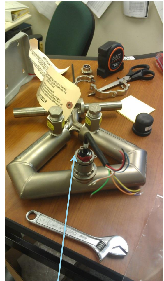
Use clip to secure connector to sensor
