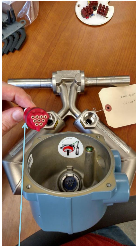
Due to o-ring, connector requires some force to pull out
