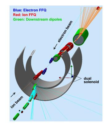
**MEIC central detector** lon beam from left at 50 mrad Electron beam from right
