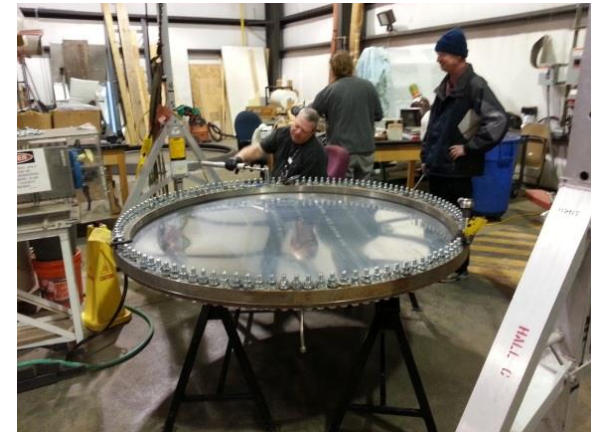
Preparation of the Vacuum Window at JLab
