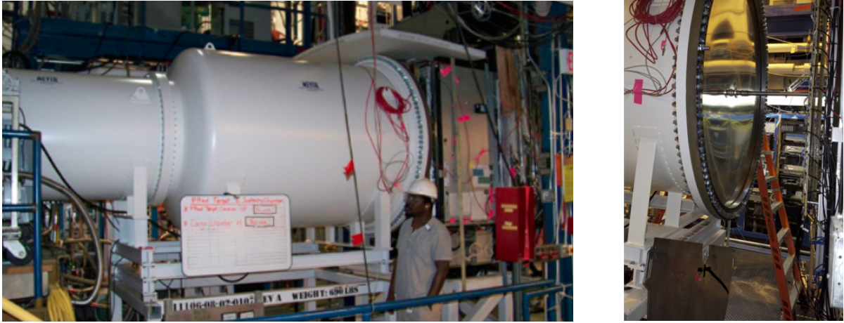
Figure 15: A photograph of the \sim 5 m long, two stage vacuum chamber used during the PRad experiment (left). A photograph of the 1.7 m diameter thin window at one end of the vacuum chamber (right). Here the GEM and HyCal have been moved downstream for technical service.
