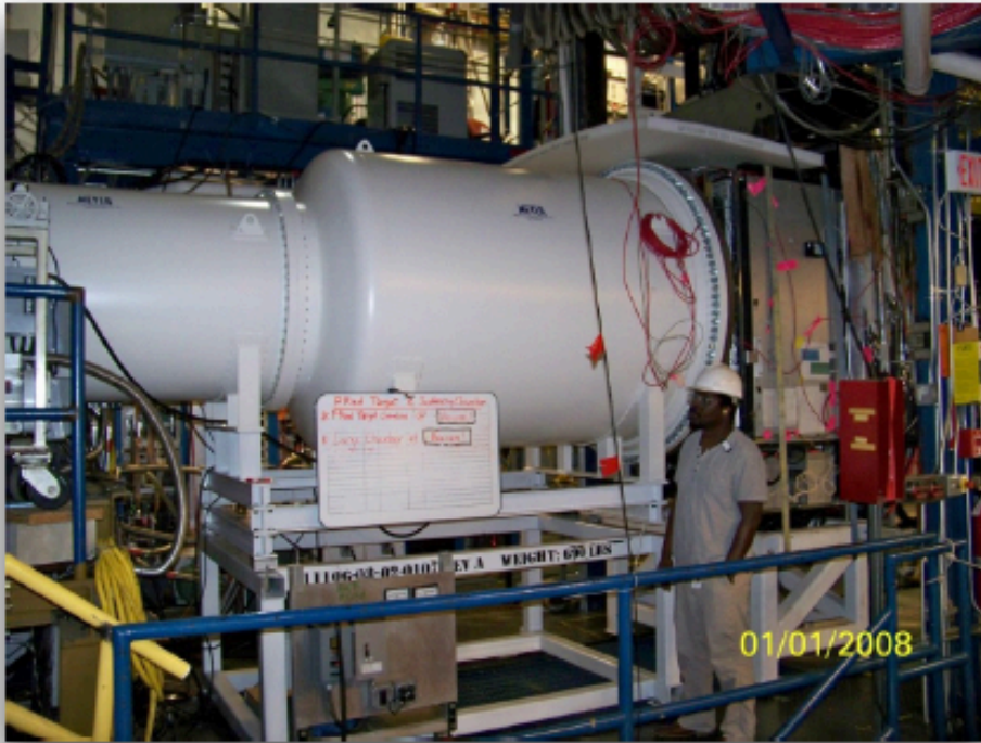
two stage, 5 m long vacuum box
