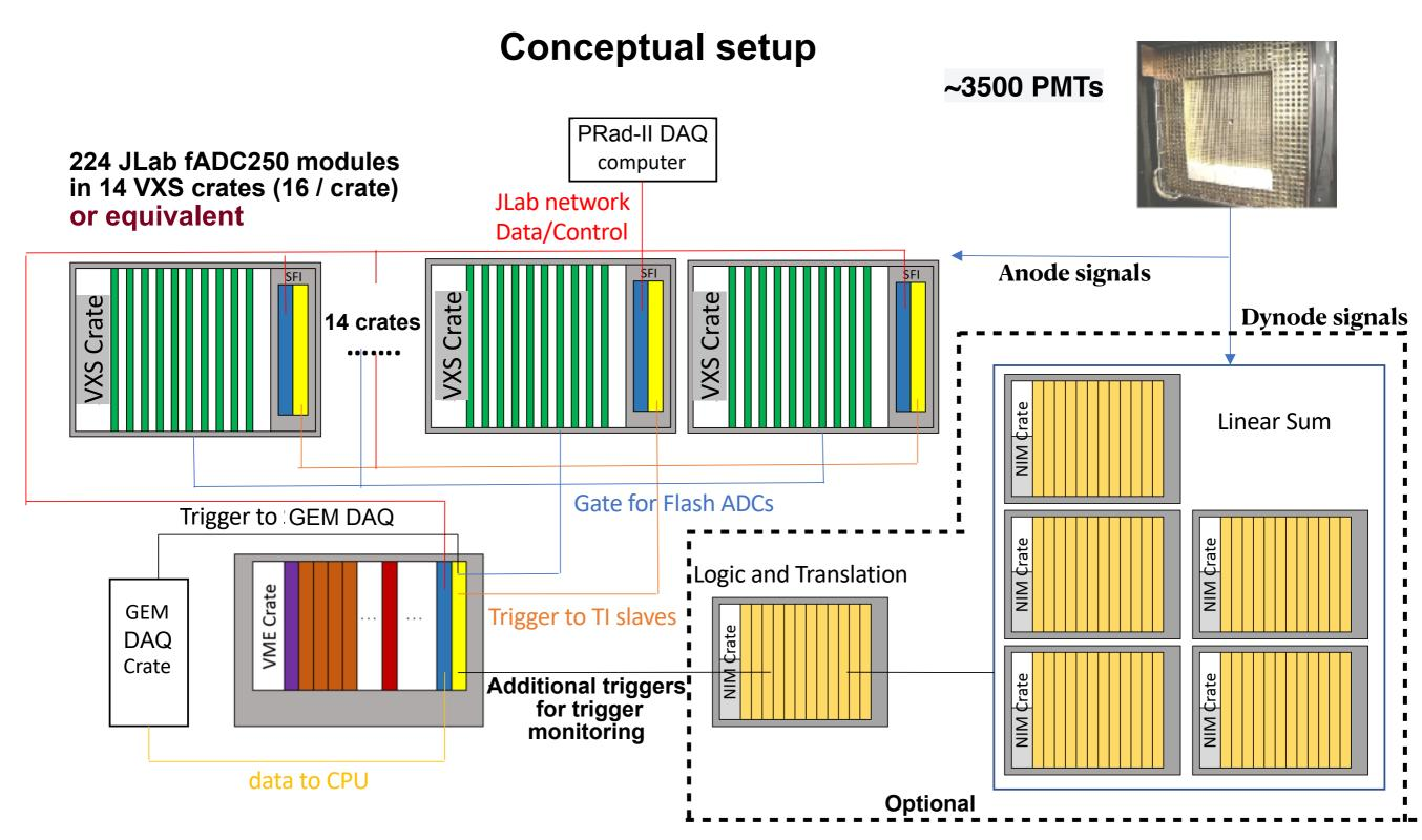
Modern flash ADC-based pipelined DAQ with robust trigger efficiency monitoring
