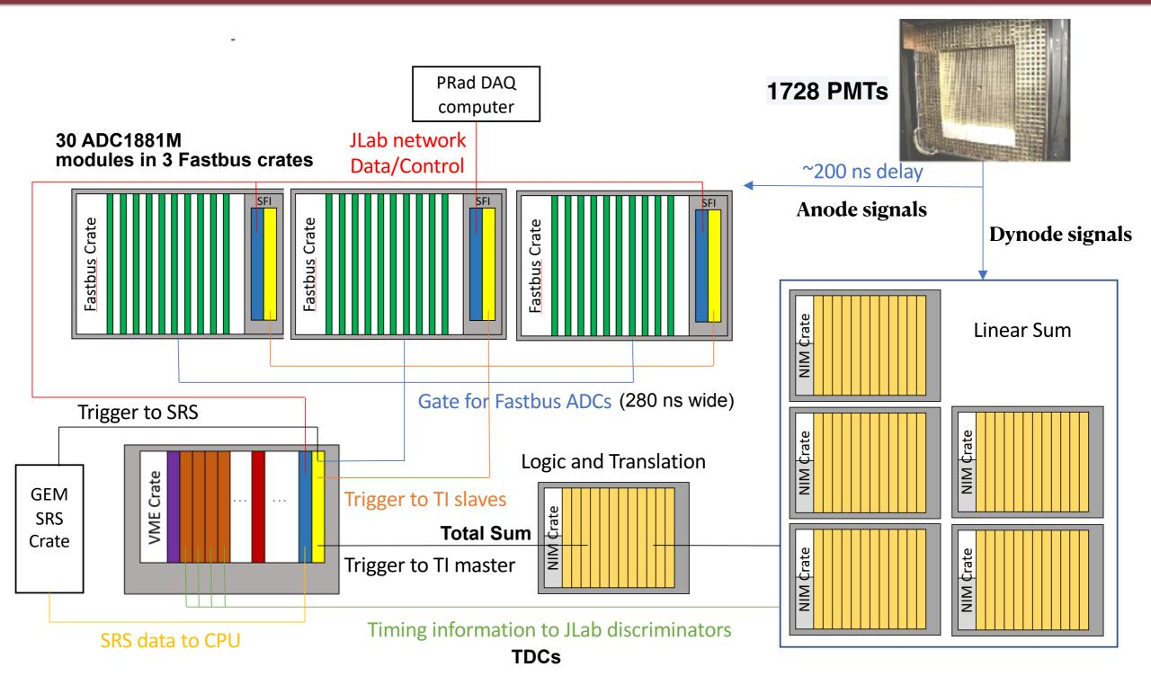
A FASTBUS-based DAQ with custom summing modules and TDCs DAQ rate ~ 4 kHz & 80-90% live-time during production.
