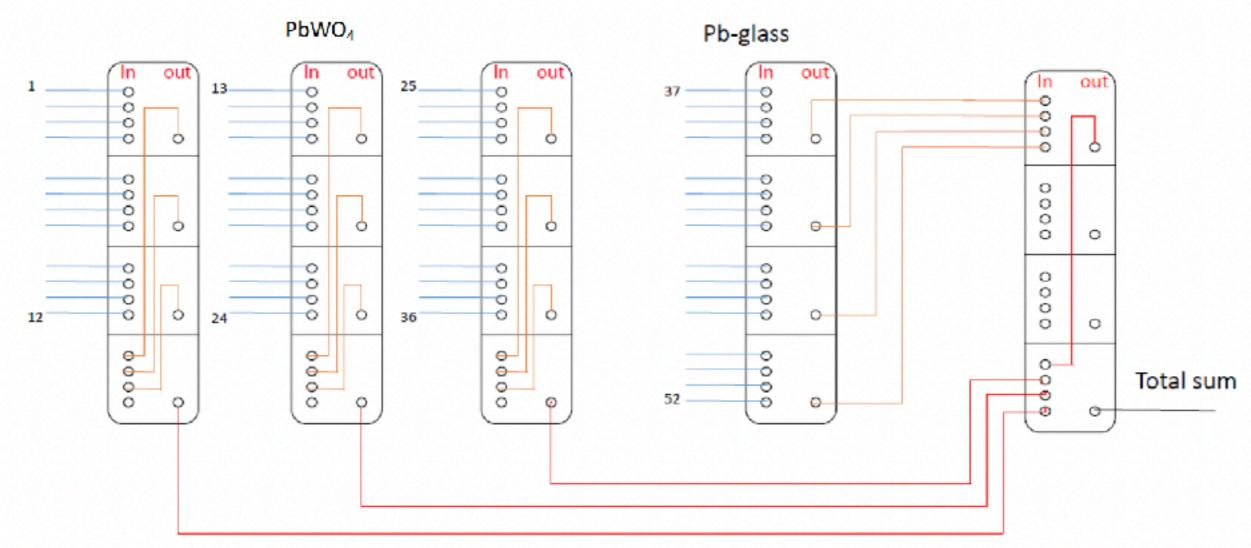
A FASTBUS-based DAQ with custom summing modules and TDCs DAQ rate ~ 4 kHz
