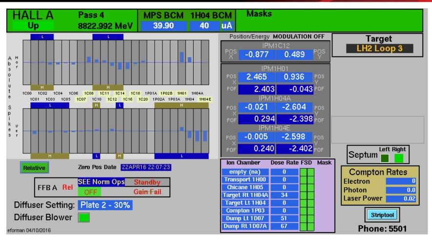
Note the 8823 MeV was used initially to set the Wien for 4<sup>th</sup> pass. The Hall A ARC measurement found the energy to be 8842 MeV.
