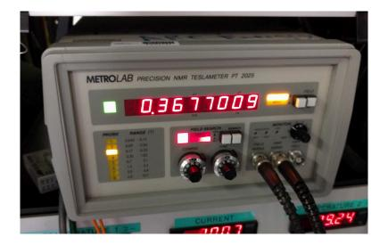
NMR can stay locked while the probe is moving through the dipole.
