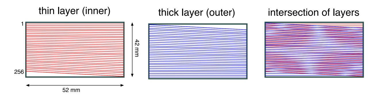
256 strips with linearly varying angles of 0 - 3 deg to minimizes dead zones. The strips will have a constant pitch of ~200 m (~1/85 deg<sup>-1</sup>). The angular resolution of  $\delta \varphi \lesssim 5$  mrad and  $\delta \theta \lesssim 10-20$  mrad.
