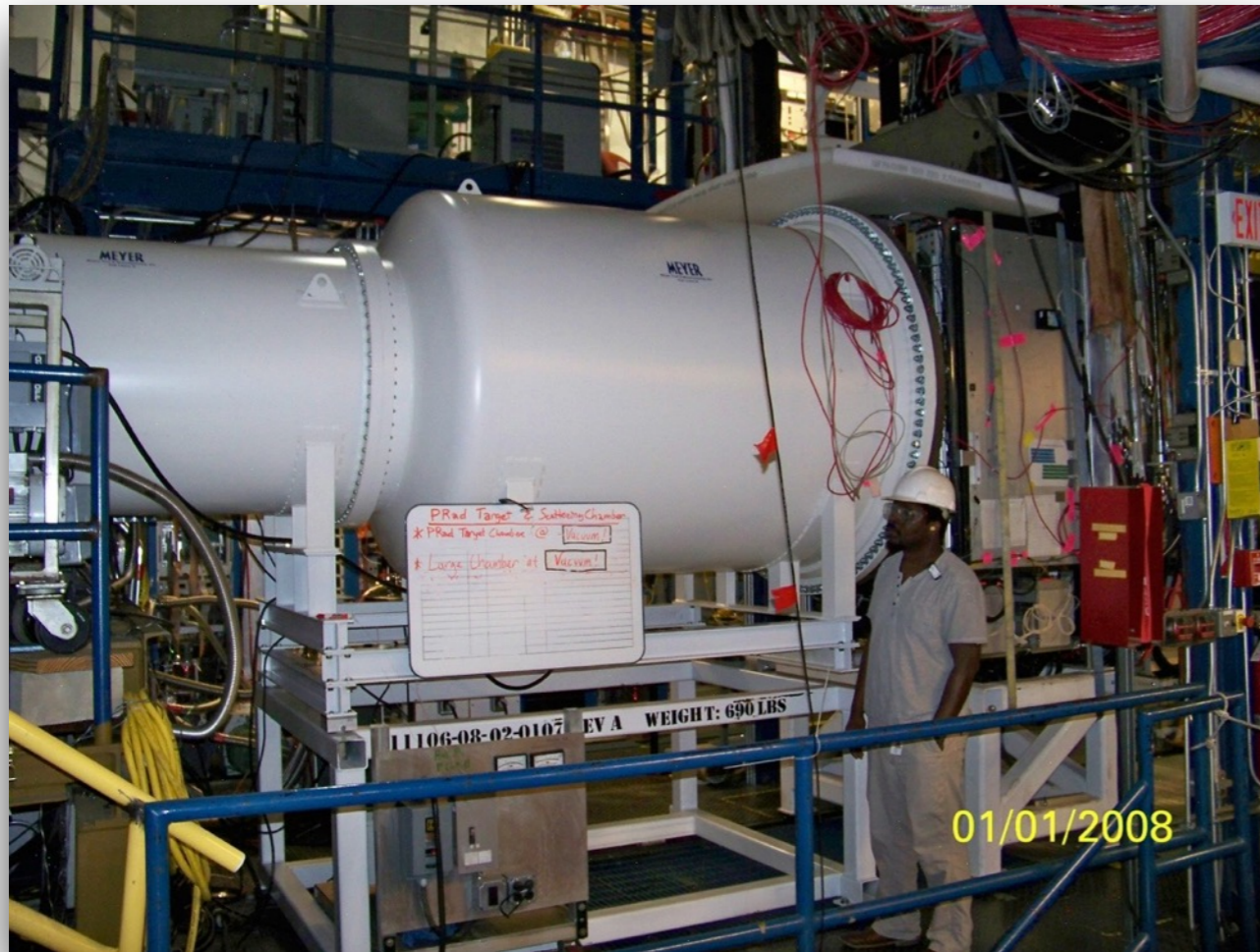
two stage, 5 m long vacuum box
