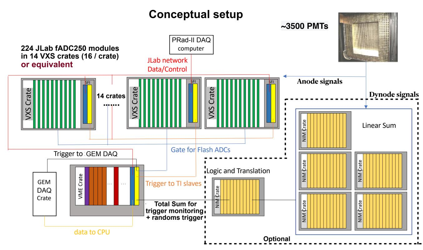
Modern flash ADC-based pipelined DAQ with robust trigger efficiency monitoring
