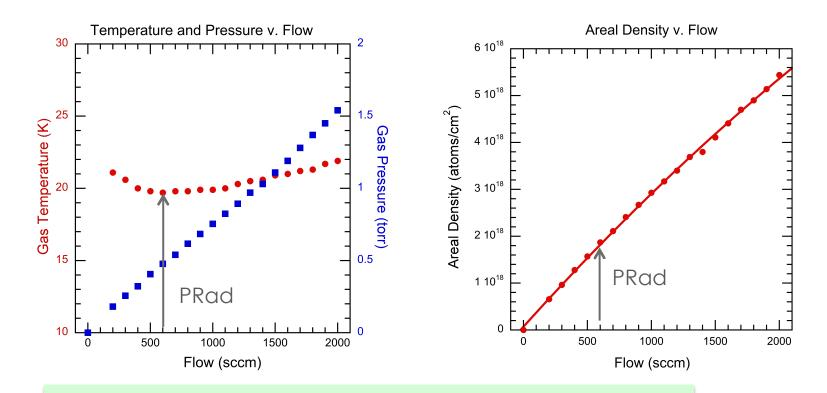
Pulse tube temperature regulated at ~15 K. H2 freezes inside fill line at lower temperature.
