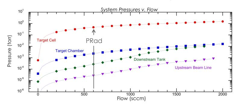
As flow increases, tank pressure converges to chamber pressure.
