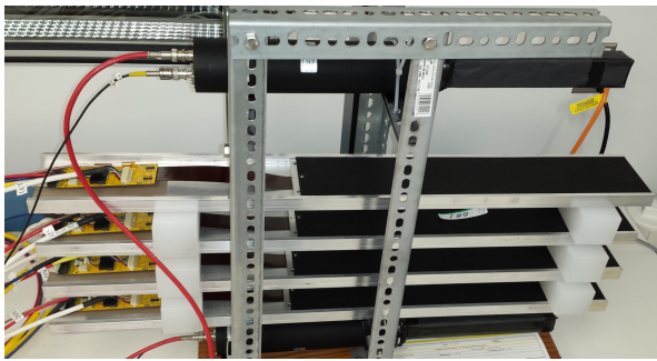
1550 Figure 86: The SVT cosmic test stand. Four SVT modules in the carrier boxes are mounted between the trigger paddles.
