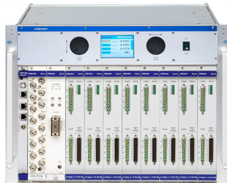
Figure 52: Wiener MPOD LX crate with mixed low and high voltage modules.
