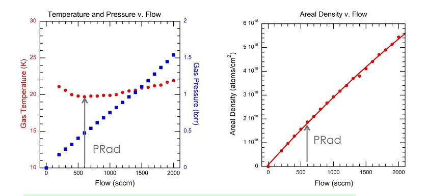
Pulse tube temperature regulated at ~15 K. H2 freezes inside fill line at lower temperature.
