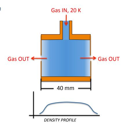
A windowless hydrogen target for Proton Charge Radius measurements in Hall B
