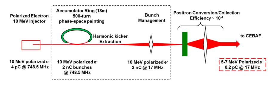
With a minimum conversion and collection efficiency of electron to positron >1E-4 using a conventional positron converter at 10 MeV the corresponding electron source conditions are 1-10 pC at 250-1000 MHz.
