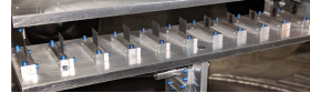
FIG. 7: Mutifoil Target for Tritium Experiment: 11 carbon foil totally which can cover the full 25cm target length
