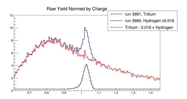
If the hydrogen contamination is in the form of H2O, we should also see Oxygen elastic peak?
