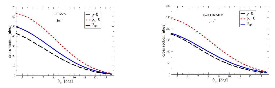
Reaction  ${}^{12}C(e, e'K^+){}^{12}{}_{\Lambda}B E_i = 3.77 \text{ GeV } E_f' = 1.56 \text{ GeV } \theta_e = 6^\circ \Phi_K = 180^\circ$ Calculations are with elementary amplitude BS3. (D. S, P. By, Phys. Rev. C 97, 025202(2018).)
