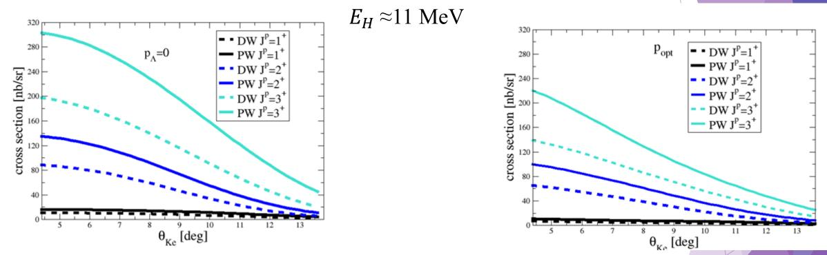
Reaction<sup>12</sup> $C(e, e'K^+)^{12}_AB E_i = 3.77 \text{ GeV } E_f' = 1.56 \text{ GeV } \theta_e = 6^\circ \Phi_K = 180^\circ$ Calculations are with elementary amplitude BS3. (D. S, P. By, Phys. Rev. C 97, 025202(2018).)
