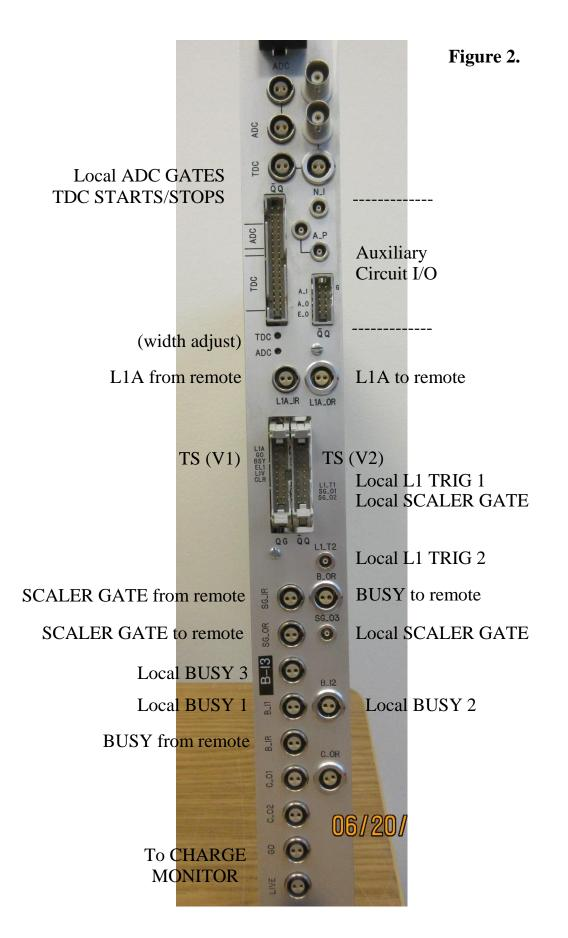
connectors. Also used are single-ended ECL levels on 50 ohm coaxial cables, and standard BNC connectors. The link to the Level 1 Trigger employs differential ECL levels on 100 ohm unshielded twisted pair cable, and a 2-pin header type connector. An additional link to the Level 1 Trigger uses NIM levels on 50 ohm coaxial cable, and a standard LEMO connector.
